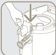
Make sure the tap handle is positioned in the tapping mechanism before the lid is closed.
