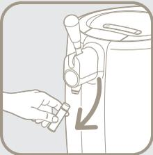
It is essential that you wash the dispensing spout before using the appliance for the first time and at least every time a new keg is connected inside the BeerTender system. This part can also be washed in a dishwasher.
