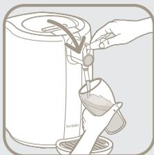
Firmly and quickly pull the handle down as far as it will go. Let the beer run into the glass.
