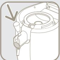
Make sure that the handle is positioned as shown on the drawing to avoid damaging the beer tube.
