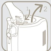
You can open the appliance by pressing the handle on top of the lid. When the handle is released, you can lift the lid up.
