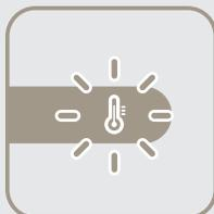
Green beer-temperature LED on the right side of the panel: when the BeerTender Keg has reached the ideal temperature the LED switches on and the appliance goes into “stand-by” cooling mode.
